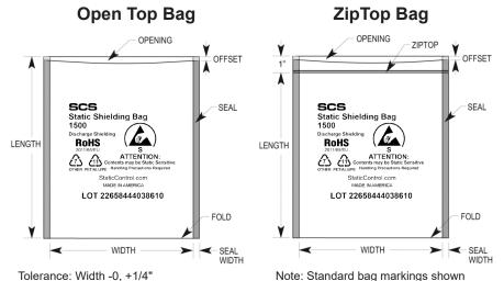
Tolerance: Width -0, +1/4" Length +/- 1/8" Offset 0 to 1/4" Seal width 3/8" with a tolerance of +/- 1/8"
