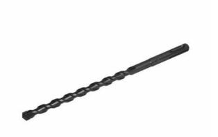
$\sim$  Tungsten carbide tipped with optimized geometry for drilling concrete and stone  $\sim$  Vacuum brazed tips for durability  $\sim$  Ground flutes designed for optimum debris removal  $\sim$  SDS-plus shank  $\sim$  Diameter: 7 mm  $\sim$  Working length: 48 mm  $\sim$  Total length: 110 mm Features & Benefits
