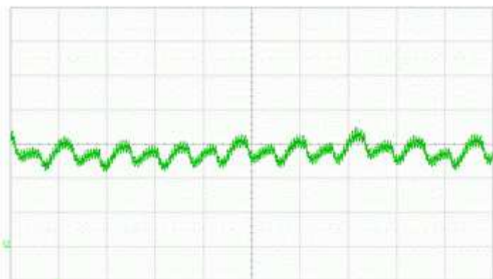
Running current @ 12 V (I = 1A/div ; t = 500ms/div)
