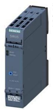
Thermistor motor prot. relay Standard evaluation unit 22.5 mm enclosure Spring-type terminals 2 CO contacts US = 24-240 V AC/DC Manual/Remote RESET with ATEX certification 2 LEDs (READY/TRIPPED) Galvanic separation Test/Reset button Open-circuit monitoring Short-circuit monitoring
