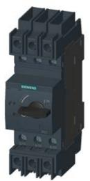
CIRCUIT-BREAKER SZ S00, FOR PLANT PROTECTION, WITH APPROBATION CIRCUIT-BREAKER UL 489. CSA C22.2 NO.5-02. A-RELEASE 1.25 A, N-RELEASE 16 A, SCREW CONNECTION, STANDARD SW. CAPACITY
