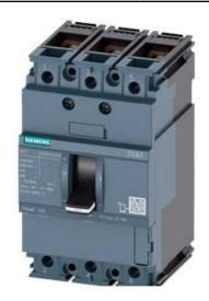
CIRCUIT BREAKER 3VA1 IEC FRAME 160 BREAKING CAPACITY CLASS H ICU=70KA @ 415 V 3-POLE, LINE PROTECTION TM210, FTFM, IN=40A OVERLOAD PROTECTION IR=40A FIXED SHORT CIRCUIT PROTECTION II=10 X IN BUSBAR CONNECTION
