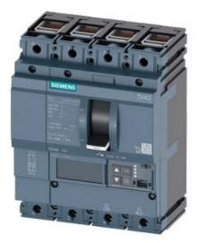
CIRCUIT BREAKER 3VA2 IEC FRAME 160 BREAKING CAPACITY CLASS M ICU=55KA @ 415 V 4POLE, LINE PROTECTION ETU550, LSI, IN=160A OVERLOAD PROTECTION IR=64A ...160A SHORT CIRCUIT PROTECTION ISD=0,6..10X IN, II=1,5..10X IN NEUTRAL PROTECTION ADJUSTABLE (OFF, UPTO 100%) CABLE CONNECTION
