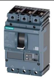
CIRCUIT BREAKER 3VA2 IEC FRAME 160 BREAKING CAPACITY CLASS M ICU=55KA @ 415 V 3POLE, LINE PROTECTION ETU560, LSIG, IN=63A OVERLOAD PROTECTION IR=25A ...63A SHORT CIRCUIT PROTECTION ISD=0,6..10X IN, II=1,5...12X IN NEUTRAL PROTECTION OPTIONAL WITH EXT. CT,UPTO 160% GROUNDFAULT, SWITCHABLE IG=0,2... 1 X IN, TG=0,050,8MS BUSBAR CONNECTION
