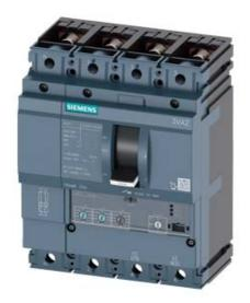
CIRCUIT BREAKER 3VA2 IEC FRAME 250 BREAKING CAPACITY CLASS L ICU=150KA @ 415 V 4POLE, LINE PROTECTION ETU320, LI, IN=160A OVERLOAD PROTECTION IR=64A ...160A SHORT CIRCUIT PROTECTION II=12 X IN NEUTRAL PROTECTION ADJUSTABLE(OFF,50%,100%) BUSBAR CONNECTION
