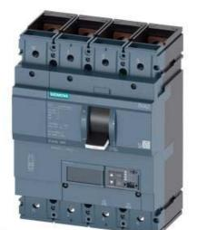
CIRCUIT BREAKER 3VA2 IEC FRAME 400 BREAKING CAPACITY CLASS C ICU=110KA @ 415 V 4-POLE, LINE PROTECTION ETU550, LSI, IN=250A OVERLOAD PROTECTION IR=100A ...250A SHORT CIRCUIT PROTECTION ISD=0,6..10X IN, II=1,5..12X IN NEUTRAL PROTECTION ADJUSTABLE (OFF, UPTO 160%) BUSBAR CONNECTION
