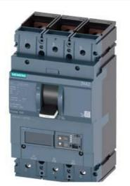
CIRCUIT BREAKER 3VA2 IEC FRAME 630 BREAKING CAPACITY CLASS M ICU=55KA @ 415 V 3-POLE, LINE PROTECTION ETU850, LSI, IN=400A OVERLOAD PROTECTION IR=160A ...400A SHORT CIRCUIT PROTECTION ISD=0,6..10X IN, II=1,5..15X IN NEUTRAL PROTECTION OPTIONAL WITH EXT. CT;UPTO 160% BUSBAR CONNECTION
