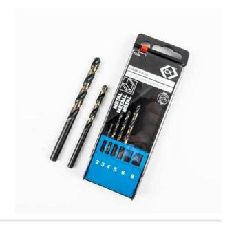
Features & Benefits  $\sim$  Cobalt Steel Flute ground Drill Set. Suitable for a range of materials including: Steel, Aluminium, Wood, Plastic, Laminated Sheet and Particle Board.  $\sim$  Set contains: 2, 3, 4, 5, 6, 8mm shank. Material: M35, cobalt steel.  $\sim$  Manufactured to DIN 338.
