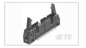
Connector System: Wire-to-Board Number of Positions: 14 Centerline (Pitch): 2.54 mm [.1 in] PCB Mount Retention: Without PCB Mount Orientation: Right Angle
