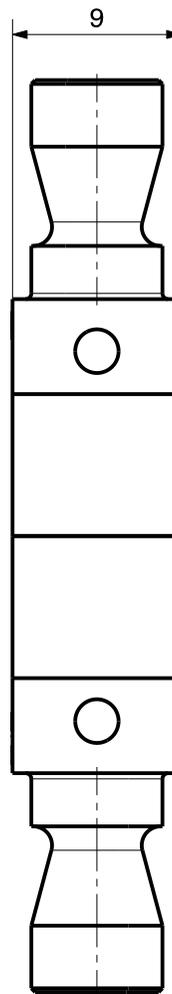
**Crimp insert for large crimp tool and table press**
