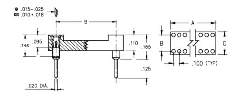
**Description:** DIP Dual In Line Socket Standard Solder Tail Open Frame Through Hole
