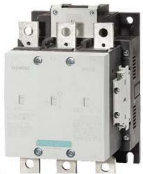
VAC. CONTACTOR, 132KW/400V/AC-3 AC(40...60HZ)/DC OPERATION UC 200-220V AUXILIARY CONTACTS 2NO+2NC 3-POLE, SIZE S10 BAR CONNECTIONS CONVENT. OPERATING MECHANISM
