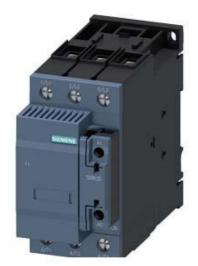
CONTACTOR, AC-6B, 50KVAR/400V, 1NO+1NC, 110V AC, 50HZ, 3-POLE, SIZE S2 SCREW TERMINAL
