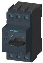
CIRCUIT-BREAKER SZ S00, FOR TRANSFORMER PROT. A-RELEASE 0.22...0.32A, N-RELEASE6.5A SCREW CONNECTION, STANDARD SW. CAPACITY
