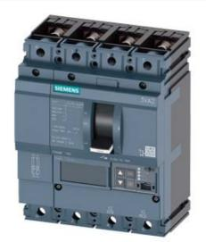
CIRCUIT BREAKER 3VA2 IEC FRAME 160 BREAKING CAPACITY CLASS L ICU=150KA @ 415 V 4POLE, LINE PROTECTION ETU550, LSI, IN=100A OVERLOAD PROTECTION IR=40A ...100A SHORT CIRCUIT PROTECTION ISD=0,6..10X IN, II=1,5..12X IN NEUTRAL PROTECTION ADJUSTABLE (OFF, UPTO 160%) BUSBAR CONNECTION
