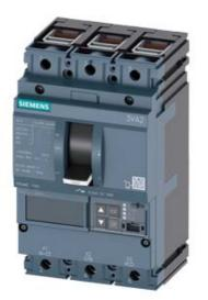
CIRCUIT BREAKER 3VA2 IEC FRAME 160 BREAKING CAPACITY CLASS L ICU=150KA @ 415 V 3POLE, LINE PROTECTION ETU560, LSIG, IN=160A OVERLOAD PROTECTION IR=64A ...160A SHORT CIRCUIT PROTECTION ISD=0,6..10X IN, II=1,5..10X IN NEUTRAL PROTECTION OPTIONAL WITH EXT. CT,UPTO 160% GROUNDFAULT, SWITCHABLE IG=0,2... 1 X IN, TG=0,050,8MS CABLE CONNECTION
