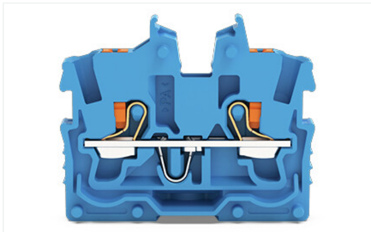
Modular terminal blocks and terminal strips with mounting flanges L = (pole no. x 3.5 mm) + 4.3 mm + 6.1 mm
