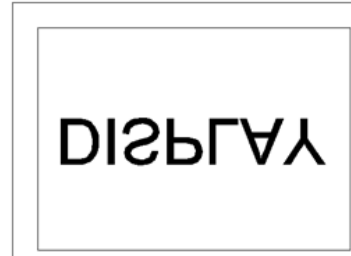
Fig. 9.9 Vertical reverse (U/D: Low; L/R: High)
