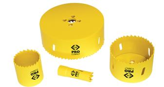
Features & Benefits ~ Premium grade 8 % Cobalt alloy steel construction for an extended working life ~ Excellent wear resistance even at high temperatures ~ For fast and clean cutting of metal, wood, aluminium, steel, cast iron, brass and plastics ~ Variable pitch teeth for rapid cutting action, efficient swarf removal and reduced vibration
