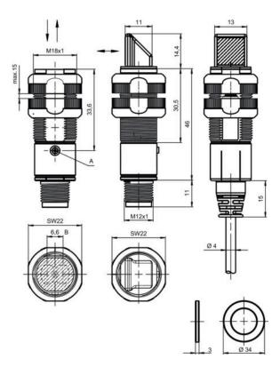
B Optical axis A Indicator diode
