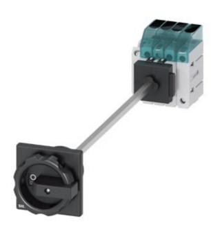
Switch disconnector 3LD3, main switch 3-polig + N, lu 63A operational switch at AC-23 A at 400 V 22,0 kW floor mounting Base mounting with door coupling center-hole 22,5 mm rotary operationg mechanism black 66 x66 mm with auxiliary 1NO+1NC
