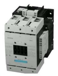
CONTACTOR, 90KW/400V/AC-3 AC(40...60HZ)/DC OPERATION UC 96-127V AUXILIARY CONTACTS 2NO+2NC 3-POLE, SIZE S6 BAR CONNECTIONS ELECTRONIC OPERATING MECHANISM WITH 24 V DC PLC INTERFACE CAGE CLAMP TERMINAL
