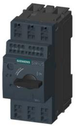
CIRCUIT-BREAKER SZ S00, FOR MOTOR PROTECTION, CLASS 10, A-RELEASE 10...16A, N-RELEASE 208A, SPRING-L. CONNECTION, STANDARD SW. CAPACITY W. TRANSVERSE AUX. SWITCH 1NO+1NC
