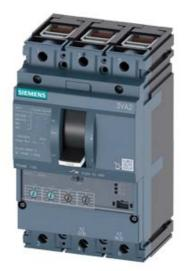
CIRCUIT BREAKER 3VA2 IEC FRAME 100 BREAKING CAPACITY CLASS H ICU=85KA @ 415 V 3POLE, LINE PROTECTION ETU330, LIG, IN=25A OVERLOAD PROTECTION IR=10A ...25A SHORT CIRCUIT PROTECTION II=1,5...12 X IN GROUNDFAULTPROTECTION IG=0,2... 1 X IN, TG=0,1/0,3MS CABLE CONNECTION
