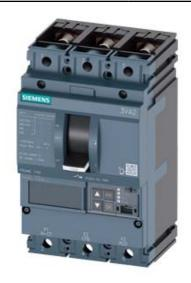
CIRCUIT BREAKER 3VA2 IEC FRAME 100 BREAKING CAPACITY CLASS H ICU=85KA @ 415 V 3POLE, LINE PROTECTION ETU860, LSIG, IN=63A OVERLOAD PROTECTION IR=25A ...63A SHORT CIRCUIT PROTECTION ISD=0,6..10X IN, II=1,5..12X IN NEUTRAL PROTECTION OPTIONAL WITH EXT. CT,UPTO 160% GROUNDFAULT, SWITCHABLE IG=0,2... 1 X IN, TG=0,050,8MS BUSBAR CONNECTION
