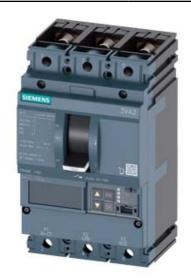
CIRCUIT BREAKER 3VA2 IEC FRAME 160 BREAKING CAPACITY CLASS L ICU=150KA @ 415 V 3POLE, LINE PROTECTION ETU860, LSIG, IN=100A OVERLOAD PROTECTION IR=40A ...100A SHORT CIRCUIT PROTECTION ISD=0,6..10X IN, II=1,5..12X IN NEUTRAL PROTECTION OPTIONAL WITH EXT. CT,UPTO 160% GROUNDFAULT, SWITCHABLE IG=0,2... 1 X IN, TG=0,050,8MS BUSBAR CONNECTION
