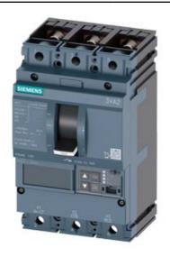
CIRCUIT BREAKER 3VA2 IEC FRAME 160 BREAKING CAPACITY CLASS M ICU=55KA @ 415 V 3POLE, LINE PROTECTION ETU560, LSIG, IN=40A OVERLOAD PROTECTION IR=16A ...40A SHORT CIRCUIT PROTECTION ISD=0,6..10X IN, II=1,5..12X IN NEUTRAL PROTECTION OPTIONAL WITH EXT. CT,UPTO 160% GROUNDFAULT, SWITCHABLE IG=0,2... 1 X IN, TG=0,050,8MS BUSBAR CONNECTION
