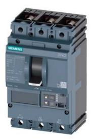
CIRCUIT BREAKER 3VA2 IEC FRAME 160 BREAKING CAPACITY CLASS M ICU=55KA @ 415 V 3POLE, LINE PROTECTION ETU860, LSIG, IN=63A OVERLOAD PROTECTION IR=25A ...63A SHORT CIRCUIT PROTECTION ISD=0,6..10X IN, II=1,5..12X IN NEUTRAL PROTECTION OPTIONAL WITH EXT. CT,UPTO 160% GROUNDFAULT, SWITCHABLE IG=0,2... 1 X IN, TG=0,050,8MS BUSBAR CONNECTION
