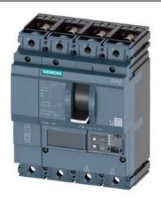
CIRCUIT BREAKER 3VA2 IEC FRAME 160 BREAKING CAPACITY CLASS H ICU=85KA @ 415 V 4POLE, LINE PROTECTION ETU860, LSIG, IN=63A OVERLOAD PROTECTION IR=25A ...63A SHORT CIRCUIT PROTECTION ISD=0,6..10X IN, II=1,5...12X IN NEUTRAL PROTECTION ADJUSTABLE (OFF, UPTO 160%) GROUNDFAULT, SWITCHABLE IG=0,2... 1 X IN, TG=0,050,8MS BUSBAR CONNECTION
