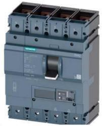
CIRCUIT BREAKER 3VA2 IEC FRAME 400 BREAKING CAPACITY CLASS C ICU=110KA @ 415 V 4-POLE, LINE PROTECTION ETU550, LSI, IN=400A OVERLOAD PROTECTION IR=160A ...400A SHORT CIRCUIT PROTECTION ISD=0,6..10X IN, II=1,5..10X IN NEUTRAL PROTECTION ADJUSTABLE (OFF, UPTO 100%) BUSBAR CONNECTION
