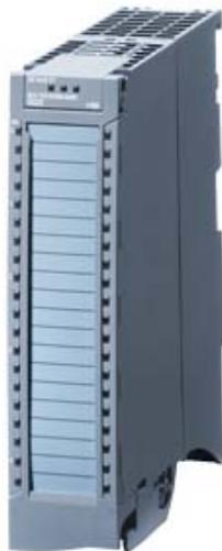
SIMATIC S7-1500, ANALOG OUTPUT MODULE AQ 4 X U/I ST; 16 BITS OF RESOLUTION, ACCURACY 0.3 %; 4 CHANNELS IN GROUPS OF 4; DIAGNOSIS, SUBSTITUTE VALUE INCL. INFEED ELEMENT, SHIELD CLAMP AND SHIELD TERMINAL
