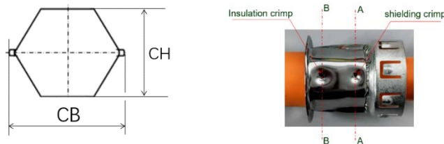
Figure 13: shielding crimp Height and Width
