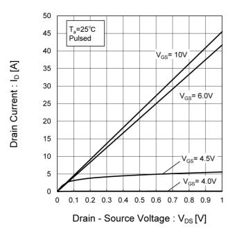
Fig.6 Typical Output Characteristics(II)
