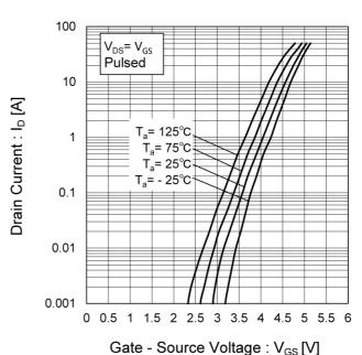
Fig.9 Gate Threshold Voltage vs.
