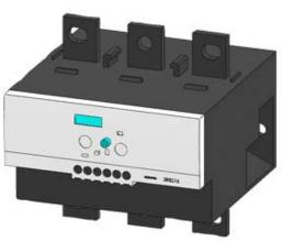
OVERLOAD RELAY 160...630 A FOR MOTOR PROTECTION SIZE S10/S12, CLASS 5...30 MOUNT. ONTO CONT./ STAND-ALONE MAIN CIRCUIT: BAR CONNECTION AUX. CIRCUIT: SCREW CONNECTION MANUAL-AUTOMATIC-RESET INT. EARTH FAULT DETECTION
