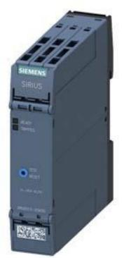
Thermistor motor prot. relay Standard evaluation unit 22.5 mm enclosure Spring-type terminals 2 CO contacts hard gold-plated US = 24 V-240 V AC/DC Manual/Auto/Remote RESET with ATEX certification 2 LEDs (READY/TRIPPED) Protective separation Test/Reset button Open-circuit monitoring Short-circuit monitoring Non-volatile
