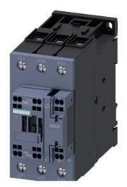
CONTACTOR,AC3:22KW/400V, 1NO+1NC, 84 - 155V AC/DC, WITH VARISTOR, 3-POLE, SIZE S2, SPRING-TYPE TERMINAL
