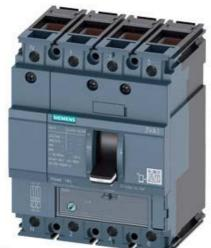
CIRCUIT BREAKER 3VA1 IEC FRAME 160 BREAKING CAPACITY CLASS N ICU=25KA @ 415 V 4-POLE, LINE PROTECTION TM220, ATFM, IN=100A OVERLOAD PROTECTION IR=70A ...100A SHORT CIRCUIT PROTECTION II=10 X IN NEUTRAL PROTECTION 100% CABLE CONNECTION
