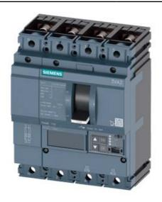
CIRCUIT BREAKER 3VA2 IEC FRAME 100 BREAKING CAPACITY CLASS C ICU=110KA @ 415 V 4POLE, LINE PROTECTION ETU560, LSIG, IN=100A OVERLOAD PROTECTION IR=40A ...100A SHORT CIRCUIT PROTECTION ISD=0,6..10X IN, II=1,5..12X IN NEUTRAL PROTECTION ADJUSTABLE (OFF, UPTO 100%) GROUNDFAULT, SWITCHABLE IG=0,2... 1 X IN, TG=0,050,8MS BUSBAR CONNECTION
