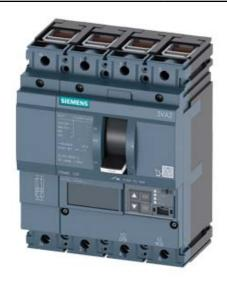
CIRCUIT BREAKER 3VA2 IEC FRAME 100 BREAKING CAPACITY CLASS H ICU=85KA @ 415 V 4POLE, LINE PROTECTION ETU860, LSIG, IN=25A OVERLOAD PROTECTION IR=10A ...25A SHORT CIRCUIT PROTECTION ISD=0,6..10X IN, II=1,5...12X IN NEUTRAL PROTECTION ADJUSTABLE (OFF, UPTO 160%) GROUNDFAULT, SWITCHABLE IG=0,2... 1 X IN, TG=0,050,8MS CABLE CONNECTION
