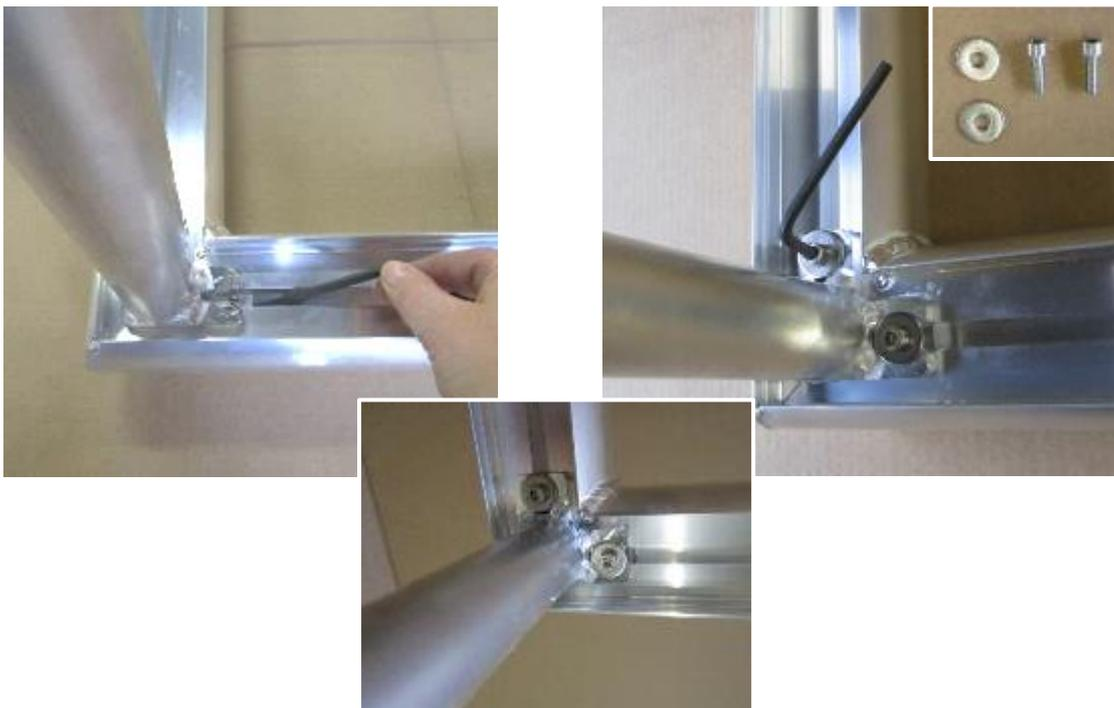
Fixing of net hoop at the bottom: At first erect the goal (see picture bottom left). Push the nut already provided in the ground frame angle below the slotted plate of the net hoop. Stick 1 washer DIN 9021, DIN 912,  $\text{\O} 7.4 \text{ mm}$  on 1 hexagon socket cylinder screw DIN 912, M6 x 20 which is then to be screwed in the nut to fix the net hoop (see picture bottom right).
