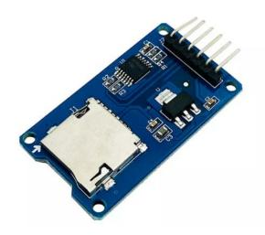
MicroSD Card Adapter can read and write files of the Micro SD card through the SPI driver program and the microcontroller system.
