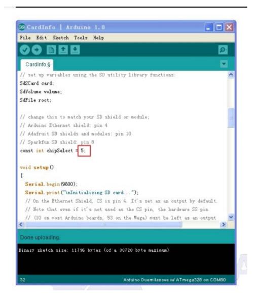
Selct serial ports, board name and click upload. This program indicates how to read the Micro SD card including about the card type, file systems, storage and file names.
