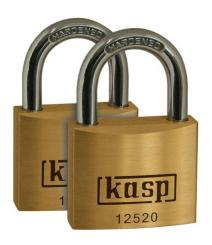
$\sim$  Hardened steel shackle  $\sim$  Solid brass body  $\sim$  Paracentric keyway  $\sim$  Padlock width: 20 mm  $\sim$  Shackle diameter: 3,5 mm  $\sim$  Internal shackle height: 12 mm  $\sim$  Pack contents: 2 padlocks with 3 keys  $\sim$  Keyed alike  $\sim$  both locks can be opened with same key Features & Benefits
