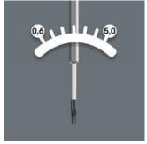
Some screw connections require specific torque values so that they can be tightened or loosened easily. Wera torque-indicators are pre-set to torque values recommended by leading carbide tool manufacturers. Pre-set torque between 0.6 Nm and 5.0 Nm, for TORX®, TORX PLUS® and hexagon socket screws, unlimited loosening torque, two handles, tamper-proof.
