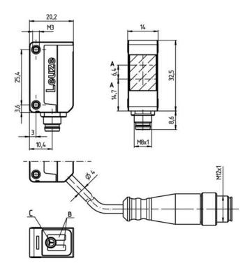
A Optical axis B Indicator diode
