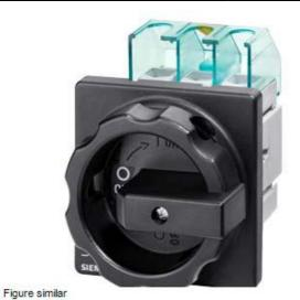
MAIN CONTROL SWITCH 3-POLE IU=100, P/AC-23A AT 400V=37KW FRONT MOUNTING FOUR-HOLE MOUNTING ROTARY ACTUATOR BLACK
