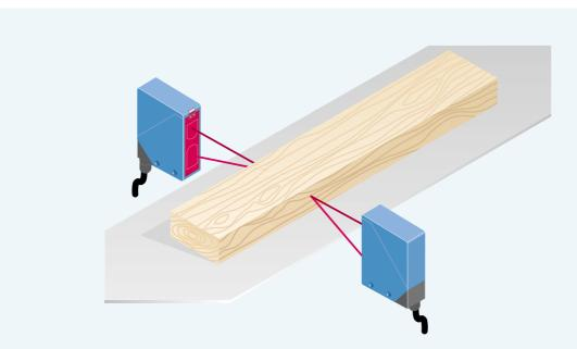
■ On circular crosscut saws, the width is measured continuously while the boards are automatically advanced. WTA 24 sensors see to this reliably.
