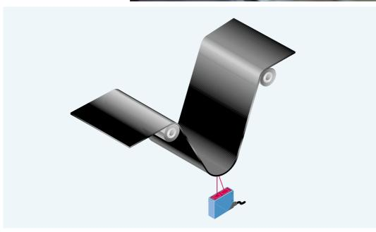
■ In continuous tyre production, supply loops regulate web tension and, therefore, the tensile force in the material. The WTA 24 ensures that the loops are fed evenly.
